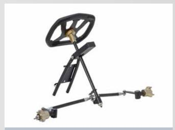
The cushioned steering column, with its guaranteed 5 cm controlled movement, allows energy to be dissipated in the event of a collision, thereby safeguarding the drivers upper limbs.
