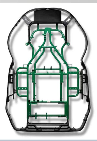
Viper E-Kart inherits the same robust safety features rigorously tested on all our rental karts. Witness the protective plastic perimeter band enveloping the chassis, shielding both driver and vital components. Plus, strategically placed polyurethane shock absorbers ensure driver and kart remain damage-free. Safety meets exhilaration!
